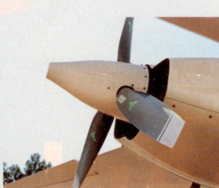
SINGLE-ENGINE performance is exceptional because the close-mounted engines, full-feathering props, and canard design make the Twin Velocity virtually incapable of spinning. Even with one engine shut down, the airplane is well mannered and easy to control (top). A three-blade MT propeller was chosen for its light weight and ground clearance (above) The spacious cabin is well appointed (left).
